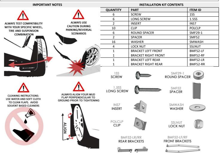
**Recommended Tools** Low-profile offset or ratcheting screwdriver, 7/16<sup>th</sup>" wrench, flathead screwdriver. **Important Tips** Installation should be done on an even surface. **Do not use power tools to tighten hardware**. **Hand tools only. Avoid overtightening**.
