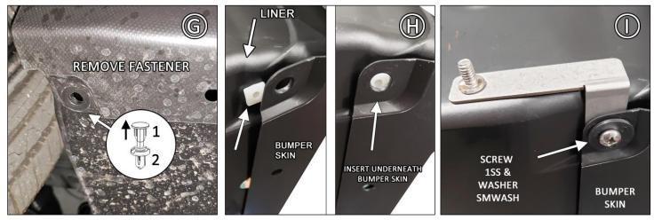
FIGURE J Install CLIP POLCLP over both mounting points on bumper.
